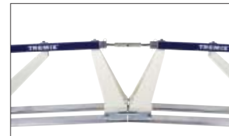
The quick couplings can be adjusted up to a +/- 5% angle to allow slopes in the slab. As an option the couplings can be replaced by a special connection for further angling up to +/-30%.
